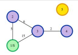
Starting at node 1, the shortest path to 2 is direct and distance 5. Going from 1 to 3, there are two paths:  $1 \rightarrow 2 \rightarrow 3$  at a distance of 5 + 6 = 11 or  $1 \rightarrow 3$  at a distance of 15. Choose the shortest path, 11. From 1 to 4, choose the shortest path through 3 and extend it:  $1 \rightarrow 2 \rightarrow 3 \rightarrow 4$  for a distance of 11 + 2 = 13 There is no route to node 5, so the distance is -1.
